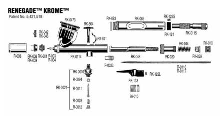
NOTE: Attached nozzle/tip housing has been permanently affixed to airbrush shell and is not made to be removed.
